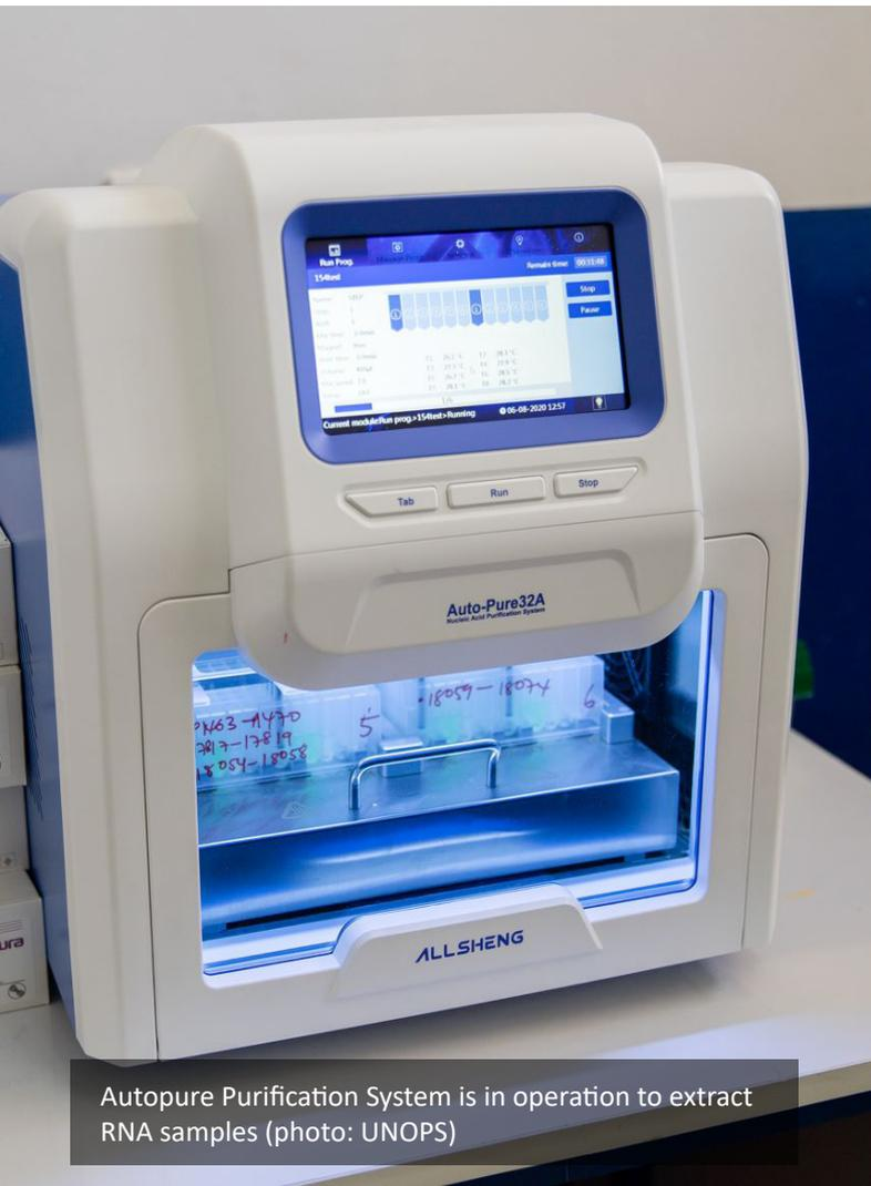
Autopure Purification System is in operation to extract RNA samples (photo: UNOPS)
