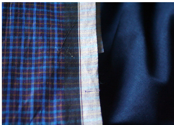
The border of a Bangladeshi lungi, showing the black & white reinforced weave border to minimize fraying
